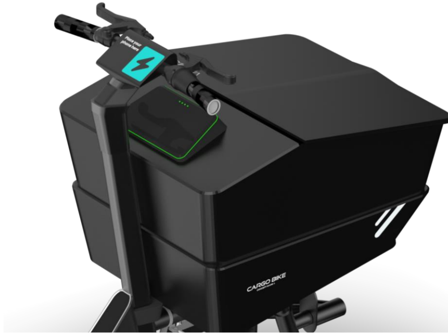
Figure 9 IoT Module highlighted in green for access control, telematics and state of charge display.
